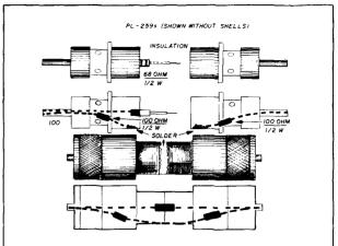
fig. 4. A 10-dB attenuator, again made from coax connectors. Three resistors form a pi network.
